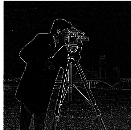
Figure 4(b). Edge detection using the combination of forward and backward differences in both directions
