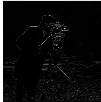
Figure 3(b). Edge detection using horizontal forward-backward difference combination
